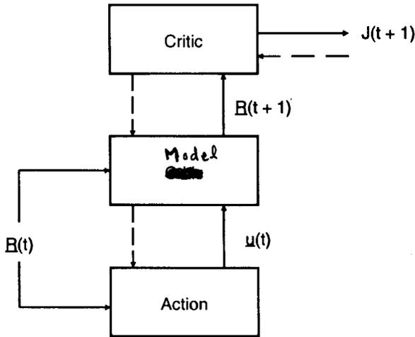
Figure 3.6 The Backpropagated Adaptive Critic (with J-style Critic).
