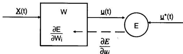
Figure 3.1 Basic backpropagation in supervised control.
