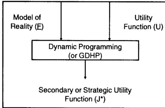
Figure 3.4 Inputs and outputs of dynamic programming.
