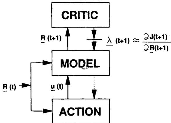
Figure 3.7 The Backpropagated Adaptive Critic (with  $\lambda$ -style Critic and  $U$  independent of  $u(t)$ ).
