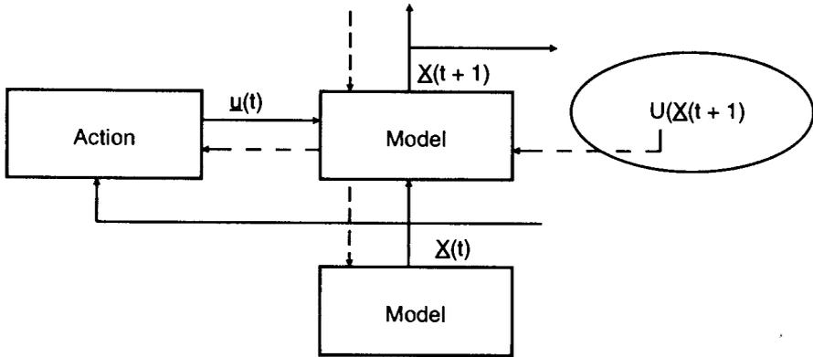
**Figure 3.3** Backpropagating utility, using backpropagation through time (BTT).
